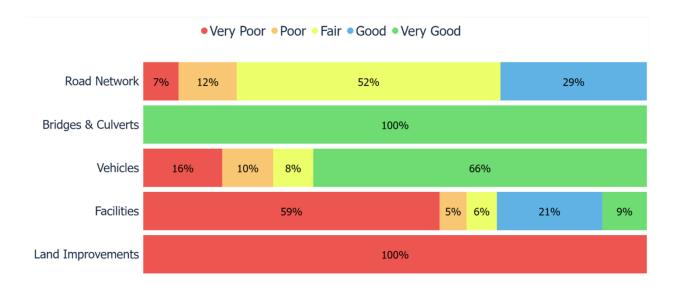
For the remaining 7% of assets, assessed condition data was unavailable, and asset age was used to approximate condition – a data gap that persists in most municipalities. Generally, age misstates the true condition of assets, making assessments essential to accurate asset management planning, and a recurring recommendation in this AMP.
